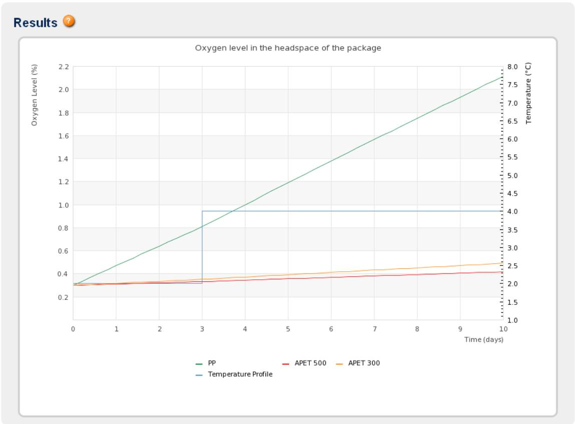
Fig. 4 PredOxyPack® output: % O<sub>2</sub> as a function of time in the headspace of a PP or PET tray with PE/EVOH/PE top film stored for 3 days at 2°C followed by 7 days at 4°C.
