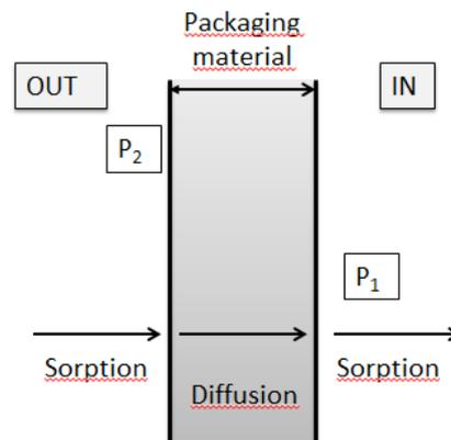
Fig. 1: Permeability model for gas transport throughout a polymer packaging material (adapted from: Robertson, 2006).  $P_1$  and  $P_2$ : partial pressure of the permeating component at respectively the inner and outer side of the packaging material
