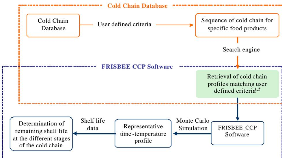
Figure 1. Illustration of FRISBEE\_CCP Software - Building of Representative Profile
