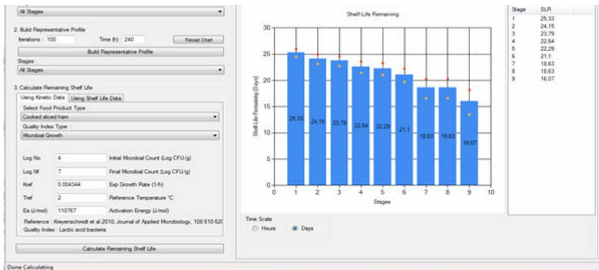
**Picture 6.** Calculated remaining shelf life of meat product at each stage of the cold chain based on a built representative profile using kinetic data (example).
